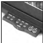
The **Yes / No** buttons allow you to confirm or deny any Advanced Feature actions. Simply press the appropriate button to answer the on-screen question posted in the **Action Bar** at the top of the Receiver's screen.
