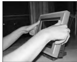
Continue to guide frame on to Receiver from top to bottom. Make sure bottom of Frame snaps on to Receiver.
