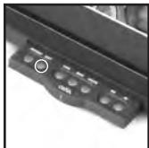
The **Next** button enables you to manually scroll through pictures in a forward direction. Press the **Next** button once to advance to the next photo. Continue to press the button until you reach the photo you are looking for. Pressing and holding the button down will resume the automatic slide show.
