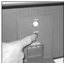
The black button on the back of the CEIVA™ Receiver adjusts the brightness setting of your screen. Pressing the black button will display a “brightness bar” on the left side of the Receiver’s screen. Press and release the black button to advance to the next setting, or to turn your CEIVA™ Receiver off. Pressing the button once, after the screen is dark, will turn the screen back on. Holding down the black button will allow you to scroll through the brightness settings.
