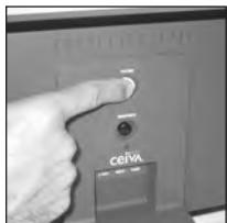
The white button on the back of the Receiver performs a variety of functions. To start the slide show, press down on the button until the message “You can let go now to start the slide show” is displayed on the screen. If you have new photos you want to view right away and don’t want to wait until the next day, simply press down on the button until the message, “You can let go now, I’m connecting” is displayed on the screen.
