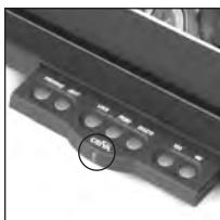
This light will glow to alert you when new pictures have been received on your CEIVA Digital Photo Receiver™. Touching any button on the Receiver will turn the light off.
