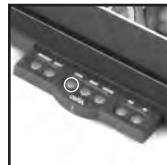
The Lock button assures that a favorite picture isn't deleted from your Receiver when new pictures are added. To lock a picture, scroll to the picture you wish to lock, then press the **Lock** button. The **Action Bar** will be displayed at the top of your Receiver's screen. Simply press the **Yes** button to **Lock** the desired
